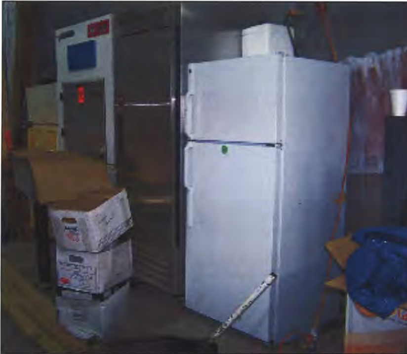
A forensic refrigerator inappropriately rigged with an extension cord was to blame for the loss of 100 rape kits.
