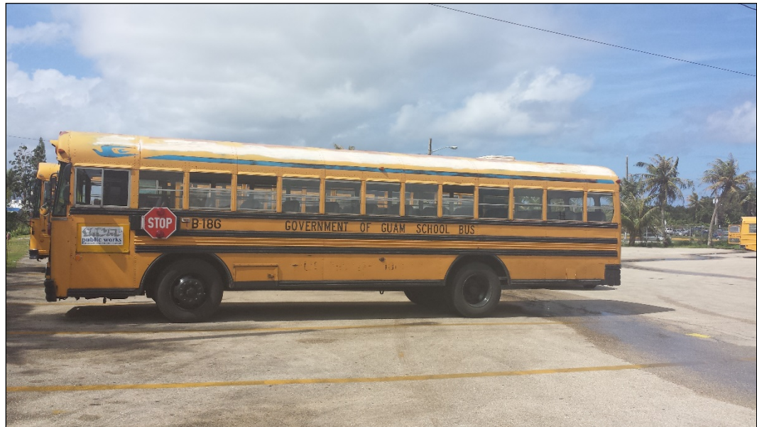
Figure 1. Older buses like this one could be replaced. Note the sun damage on roof and the rust spots. Source: Office of Inspector General.
