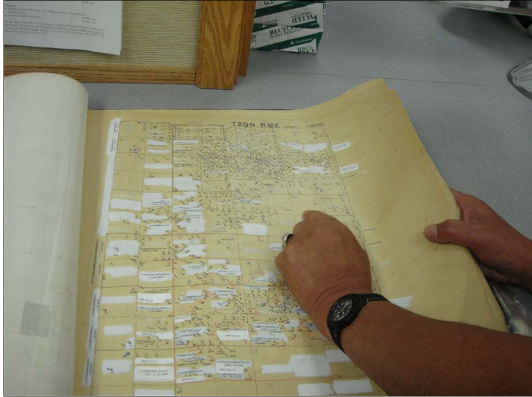
Figure 1. Linen plat map used to identify well locations and help maintain lease information.
