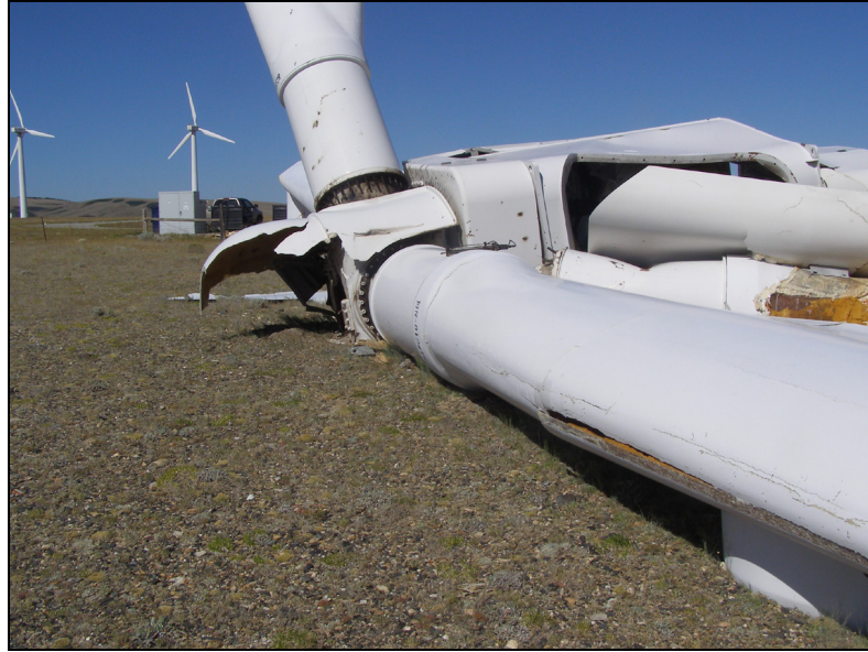
Figure 3. Collapsed 600 kilowatt turbine on BLM wind project in Wyoming that went unreported for several weeks. Source: BLM.
